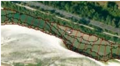
Figure 7. Examples of segmentation polygons (in black) and disaggregated Geographic Object (in red).
