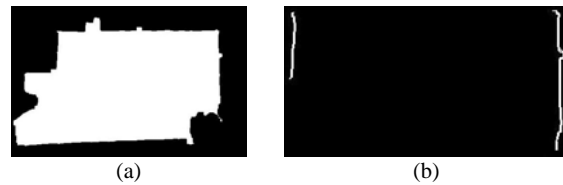
Figure 2. (a) The final segmented region and (b) the vertical lines detected through Hough transform
