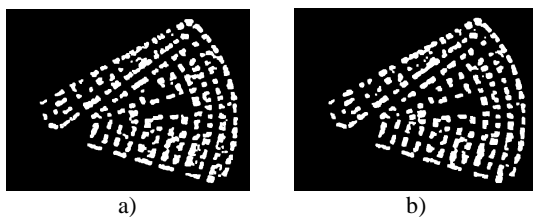
Figure 5: a) Raw segmented roof-tile spots; b) Raw building extraction results with Feature Analyst software (Santos et al., 2009)
