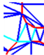
(a) Triangle edge filtering based on proximity. Shortest edges closing gaps are kept. Cyan edges are kept, blue edges are deleted.
