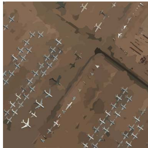
(b) Segmentation result at LOD = 5. Number of produced polygons = 884.
