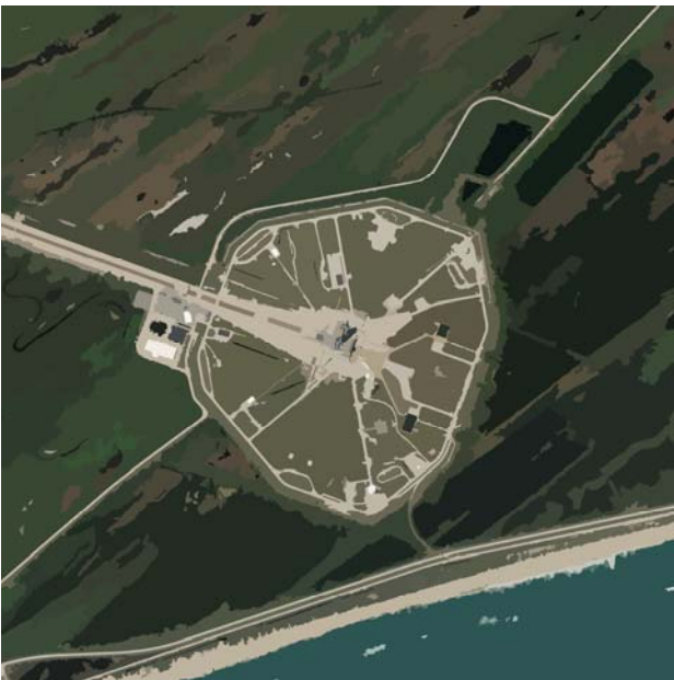
(b) Result of the image segmentation on the 12th LOD. The number of constructed polygons is 602. Each polygon is attributed with the colour averaged over the colours of the pixels covered by polygon. Data reduction factor (number of pixels divided by number of polygons) is 13,912. Triangulation tessellation generated by the Constrained Delaunay triangulation over the edge set contained 1,722,514 triangles.
